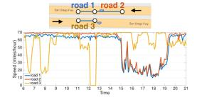
Figure 1: Spatial correlation is dominated by road network structure. (1) Traffic speed in road 1 are similar to road 2 as they locate in the same highway. (2) Road 1 and road 3 locate in the opposite directions of the highway. Though close to each other in the Euclidean space, their road network distance is large, and their traffic speeds differ significantly.
