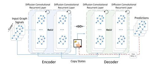
Figure 2: System architecture for the *Diffusion Convolutional Recurrent Neural Network* designed for spatiotemporal traffic forecasting. The historical time series are fed into an encoder whose final states are used to initialize the decoder. The decoder makes predictions based on either previous ground truth or the model output.
